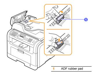
Insert a new ADF rubber pad into place.
